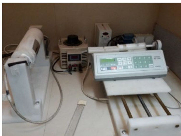
Fig. 1. The electrospinning machine in nanotechnology and advanced materials institute.
