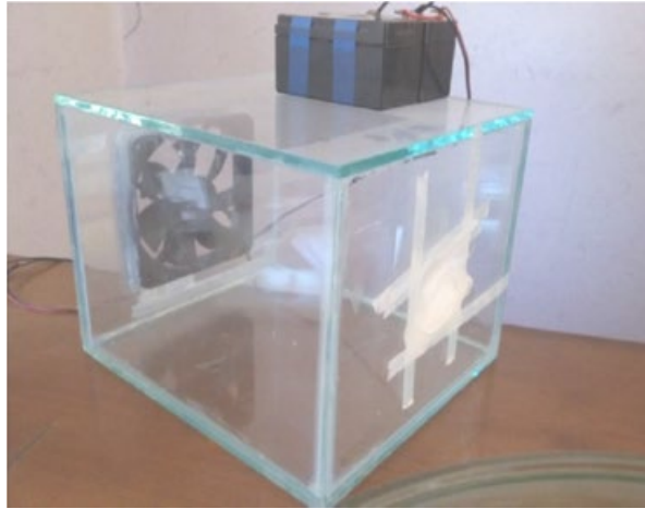
Fig. 2. The device fabricated for stabilization of membrane and NO x removal test.
