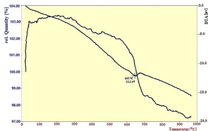
Fig. 2. TGA and DTA curves of Sm 2 O 3 NPs
