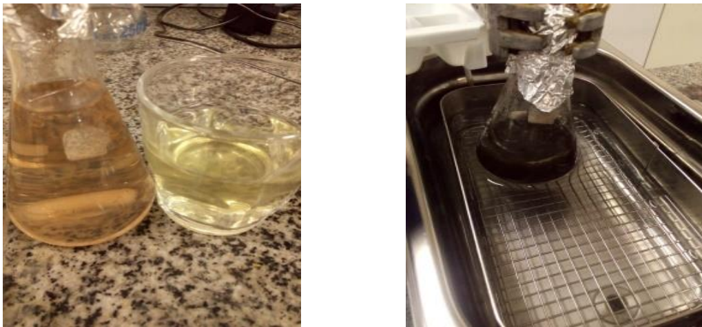
Fig. 2. Pictures of silver nanoparticle synthesis steps are:(A) 10 mL of viscum album fruit extract and 50 mL of 10 mM aqueous silver nitrate solution, after 30 min.(B) 30 mL of extract with 10 mM aqueous silver nitrate solutions after 2 h under ultrasonic.
