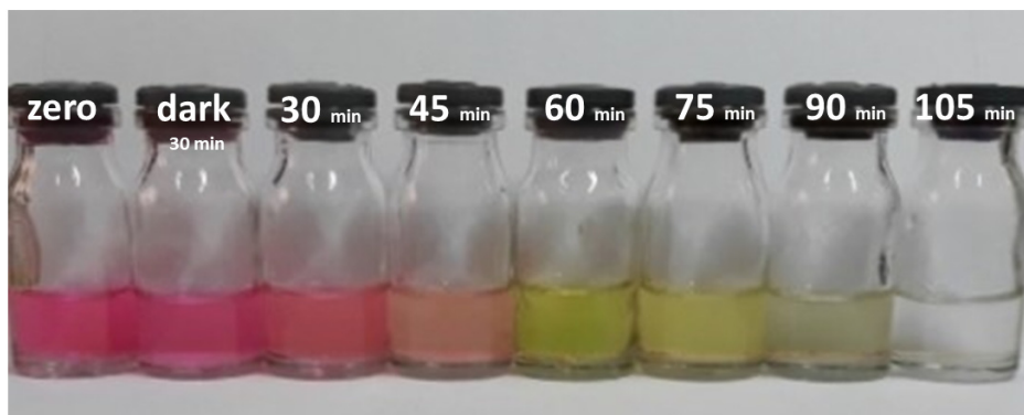
Fig. 11. Color change of the RhB solution under visible light irradiation and in the presence of N -TiO 2 /C. Measurement conditions: 40 mg photocatalyst, 40 mL RhB aqueous solution containing 10 ppm of RhB, and a light source of 40-Watt white LED lamp
