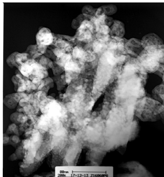
Fig. 6: TEM image of Ir-doped TiO 2 NPs
