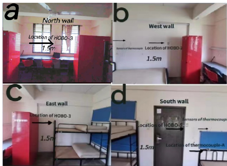
Fig. 6. Images of (a) installation of equipment on the north wall; (b) installation of equipment on the west wall; (c) installation of equipment on the east wall; (d) installation of equipment on the south wall
