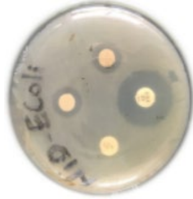
Fig. 10. Lawn culture of E. coli indicating zone of inhibition around NiO nanoparticle coated discs and standard antibiotic discs after 18 hrs of incubation at 37 °C
